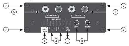
TSD Input/Output connections are removable for easy system wiring. The connectors have a 3.5mm pitch between pins.
